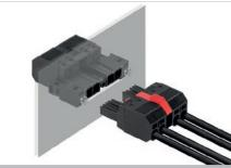
180° inverted male header featuring PUSH IN connection technology for field wiring in 6 mm<sup>2</sup> with a 7.62 pitch as a "three-flange variant" for enclosure feed-throughs. Suitable for enclosures with a max. wall thickness of 16 mm. Also a perfect finger-safe solution for reverse voltages. Meets the requirements of UL1059 600 V Class C and IEC 61800-5-1.
