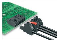
Male header with 90° outlet direction and optional solder flange with leading PE contact. Enables UL approval for 600 V in accordance with UL61800-5-1 / UL840. In combination with the female plug BUZ 10.16 IT meets the enhanced requirements for 5.5 mm of touch safety on IT power networks in acc. with IEC 61800-5-1 for 400 V relative to earth. Even when no female plug is present, the mating profile ensures that at least >1 mm of touch safety is present with a finger pressure of 20 N.
