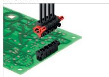
Female plug with clamping yoke screw connection in 180° outlet direction. Complies with UL1059 600 V Use Group C and IEC 61800-5-1 requirements for 3 mm of finger safety on 400 V TNC(S) systems.
