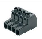
Male plug in 180° outlet direction with clamping yoke screw connection for TNC (S) systems. Meets the requirements of UL1059 for 600 V Use Group C. The mating profile ensures touch safety of more than 3 mm according to IEC 61800-5-1 when connected.
