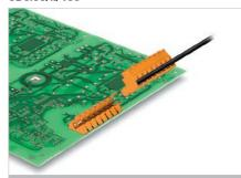
Male headers with 135° wire outlet, optimised for wave soldering. Available in versions with either open or closed ends (B). Mounting blocks can be attached onto the closed variants. The blocks can be used to screw on to the female plug of the circuit board. The male headers can be manually coded or ordered as pre-coded headers.
