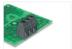
High-power PCB Terminal with clamping yoke screw connection, in 10.16 mm pitch for wire cross-sections up to 16 mm<sup>2</sup> (AWG 6).
