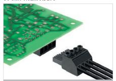
Male header with 270° outlet direction for 400 V TNC(S) systems. Enables UL approval for 600 V in accordance with UL61800-5-1 / UL840. The pin arrangement ensures finger safety of >3 mm in accordance with IEC 61800-5-1. Maximum operational reliability thanks to derating up to 125°C, a 100% failsafe pin arrangement, unique coding diversity and additional fastening.
