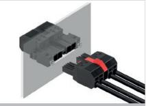
180° inverted male header featuring PUSH IN connection technology for field wiring in 6 mm<sup>2</sup> with a 7.62 pitch as a "three-flange variant" for enclosure feed-throughs. Suitable for enclosures with a max. wall thickness of 2 mm. Also a perfect finger-safe solution for reverse voltages. Meets the requirements of UL1059 600 V Class C and IEC 61800-5-1.
