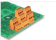
Multi-level PCB terminal with our proven clamping yoke screw connection in 5.08 mm pitch, suitable for wire cross-sections up to 2.5 mm².
