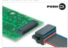
Female plug provides pluggable connection level with common minus (PNP sensor) for decentralized I/O electronics with integrated LED display; used together with male headers in 3.5 mm pitch. Available with a screw flange (F) or a lock an release lever (LR).
