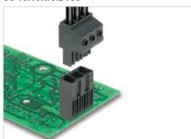
Male header with 180° outlet direction for TNC(S) systems. Enables UL approval for 600 V in accordance with UL61800-5-1 / UL840. The pin arrangement ensures more than 3 mm of touch-safety in acc. with IEC 61800-5-1.
