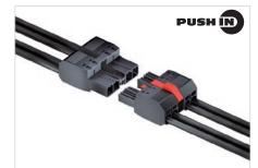
Male plug in 180° outlet direction with PUSH IN spring connection for TNC(S) networks. Also perfect for finger-safe solutions involving inverse voltages. Meets the requirements of UL1059 for 600 V Use Group C. The mating profile ensures touch-safety of > 3 mm in accordance with IEC 61800-5-1.
