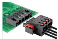
Female plug in 180° outlet direction with clamping yoke screw connection for TNC (S) systems. Meets the requirements of UL1059 for 600 V Use Group C. Ensures touch-safety of
