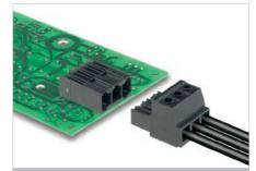
Male header with 90° outlet direction for 400 V TNC(S) systems. Enables UL approval for 600 V in accordance with UL61800-5-1 / UL840. The pin arrangement ensures more than 3 mm of touch-safety in acc. with IEC 61800-5-1.
