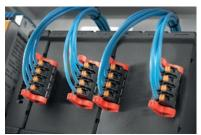
The solder flange solution for the pin connector on the PCB and the possible flange fixing of the plug section simplify the use of complex device applications with high mechanical demands
