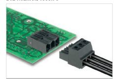
Female plug in 180° outlet direction with clamping yoke screw connection and additional shield connection for TNC (S) systems. Meets the requirements of UL1059 for 600 V Use Group C. The mating profile ensures touchsafety of > 3 mm in accordance with IEC 61800-5-1.
