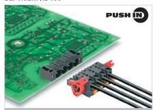
Female plug with PUSH IN spring connection in 180  $^{\circ}$  outlet direction. Complies with UL1059 600 V Use Group C and IEC 61800-5-1 requirements for 3 mm of finger safety on 400 V TNC(S) systems.
