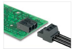
Male header with 90° outlet direction for 400 V TNC(S) systems. Enables UL approval for 600 V in accordance with UL61800-5-1 / UL840. The pin arrangement ensures more than 3 mm of finger safety in accordance with IEC 61800-5-1.
