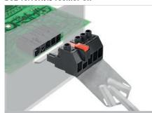
Female plug with 180° outlet direction for IT power networks. Meets the requirements of UL1059 for 600 V Use Group C. Leading PE contact in combination with the male header SU 7.62 IT. Meets the enhanced requirements for 5.5 mm of touch safety on IT power networks in acc. with IEC 61800-5-1 for 400 V relative to earth. The self-locking middle flange which can also be optionally screwed, reduces the space requirements by one pitch width compared to conventional solutions.
