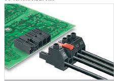
Male header with 270° outlet direction for TNC(S) systems. Enables UL approval for 600 V in accordance with UL61800-5-1 / UL840. The pin arrangement ensures more than 3 mm of touch-safety in acc. with IEC 61800-5-1.
