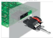
Hybrid female connector with power and signal contacts and adjustable actuator (pusher) featuring PUSH IN spring connection technology. Enables simultaneous connection of power, signals and shielding. Ideal for connecting servo and asynchronous drives. Meets the requirements of UL1059 for 600 V Use Group C. The pin arrangement guarantees more than 3 mm of touch-safety in accordance with IEC 61800-5-1. The snap-on middle flange decreases the space required by one pitch width.
