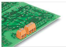
Highly compact PCB terminal with leaf spring screw connection in 3.5 mm pitch for wire cross-sections up to 1.5 mm<sup>2</sup>.
