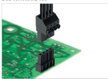
Finger-safe female header with 180° outlet direction for PCBs. Meets the requirements of IEC 61800-5-1 and allows UL approval in accordance with UL508 / UL840 for 600 V. An ideal finger-safe solution for power output and DC-link applications. The pin arrangement is finger-safe. The assembly coding ensures that it cannot be assembled on the PCB turned
