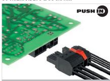
Hybrid male header with 270° outlet direction with power and signal contacts. Meets the enhanced requirements for 3 mm of touch safety for 400 V TNC(S) systems in acc. with IEC 61800-5-1 and comes with UL approval for 600 V in acc. with UL508-5-1 / UL840.
