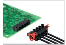
Male header with 90° outlet direction. The compact and efficient solution for UL-600 V applications in the lower power range in combination with a female plug fulfils the requirements for 600 V acc. to UL508 / UL840 and the enhanced electric shock protection requirements acc. to IEC 68100-5-1.
