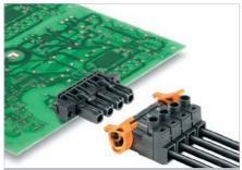
Touch-safe female header with 90° outlet direction for PCBs. Meets the requirements of IEC 61800-5-1 and comes with UL approval in accordance with UL508-5-1 / UL840 for 600 V. An ideal touch-safe solution for power output and DC-link applications. The pin arrangement ensures more than 3 mm of touch-safety in accordance with IEC 61800-5-1.
