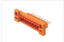
Feed-through male connector with optional locking function, for mounting on front plate. Internal connection as flat-blade or solder connection. All male headers can be manually coded or ordered as pre-coded headers.
