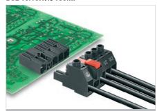
Female plug with 180° outlet direction for IT power networks. Meets the requirements of UL1059 for 600 V Use Group C. Leading PE contact in combination with the male header SU 7.62 IT. Meets the enhanced requirements for 5.5 mm of touch safety on IT power networks in acc. with IEC 61800-5-1 for 400 V relative to earth.
