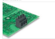
High-power PCB Terminal with clamping yoke screw connection, in 15.00 mm pitch for wire cross-sections up to 50 mm<sup>2</sup> (AWG 1).
