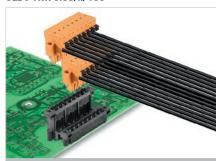
Double-level, high-temperature-resistant male header, optimised for SMT processing. The connection levels are offset and designed for a female plug with screw connection or PUSH IN wire connect. The male headers can be manually coded or ordered as pre-coded headers.
