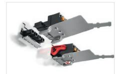
$180^\circ$  inverted male header with PUSH IN connection technology for field wiring in 2.5 mm² with a 7.62 pitch. Also ideal as a touch-safe solution for inverse voltages. Meets the requirements of UL1059 600 V class C and IEC 61800-5-1.
