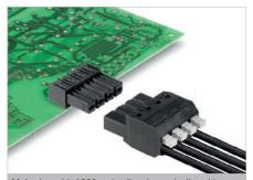
Male plug with 180° outlet direction and adjustable actuator (PUSHER) featuring PUSH IN spring connection technology for TNC(S) networks. Also perfect as a touch-safe solution for reverse voltages. Meets the requirements of UL1059 for 600 V Use Group C. The pin arrangement ensures finger-safety of >3 mm in accordance with IEC 61800-5-1.
