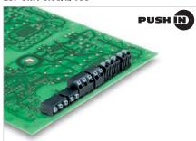
PCB terminal for fully automatic assembly in 5.00 mm pitch, for THR reflow soldering (SMT) and wave soldering.
