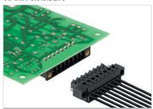
High-temperature-resistant male header with 270° plugging angle (the angle between the plugging direction and the solder pin). This angle has a plugging direction that is parallel to the circuit board with female plugs plugged in upside down.
