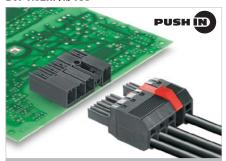
Female plug in 180° outlet direction with PUSH IN spring connection for TNC (S) systems. Meets the requirements of UL1059 for 600 V Use Group C. The mating profile ensures touch-safety of > 3 mm in accordance with IEC 61800-5-1.
