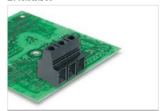
High-power PCB Terminal with clamping yoke screw connection, in 15.00 mm pitch for wire cross-sections up to 25 mm<sup>2</sup> (AWG 4).
