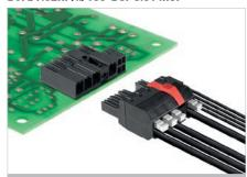
Hybrid female connector with power and signal contacts and adjustable actuator (pusher) featuring PUSH IN spring connection technology. Enables simultaneous connection of power, signals and shielding. Ideal for connecting servo and asynchronous drives. Meets the requirements of UL1059 for 600 V Use Group C. The pin arrangement guarantees more than 3 mm of touch-safety in accordance with IEC 61800-5-1. The snap-on middle flange decreases the space required by one pitch width.
