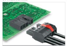
Male header with 90° outlet direction for 400 V TNC(S) systems. Enables UL approval for 600 V in accordance with UL61800-5-1 / UL840. The pin arrangement ensures more than 3 mm of touch-safety in acc. with IEC 61800-5-1.
