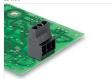
High-power PCB terminal with proven clamping yoke screw connection, 6.35 mm pitch, for conductor crosssections up to 6 mm<sup>2</sup>.
