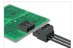
Male header with 90° outlet direction for TNC(S) systems. Enables UL approval for 600 V in accordance with UL61800-5-1 / UL840. The pin arrangement ensures more than 3 mm of touch-safety in acc. with IEC 61800-5-1.
