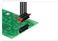
Pin header with 270° outlet direction. This compact solution for UL-600 V applications in the lower performance range meets the requirements for 600 V in accordance with UL 508 / UL 840 as well as the more stringent touch-safety requirements of IEC 68100-5-1 for electrical drive systems when combined with a female plug.
