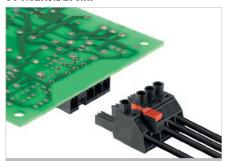
Male header with 270° outlet direction with a leading PE contact for IT power networks. Enables UL approval for 600 V in accordance with UL61800-5-1 / UL840. In combination with the female plug BVZ 7.62 IT meets the enhanced requirements for 5.5 mm of touch safety for IT power networks in acc. with IEC 61800-5-1 for 400 V relative to earth. Even when no female plug is present, the mating profile ensures that at least >1 mm of touch safety is present with a finger pressure of 20 N.
