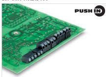
PCB terminal for fully automatic assembly in 7.62 mm pitch, for THR reflow soldering (SMT) and wave soldering.
