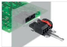
Hybrid female connector with power and signal contacts with PUSH IN spring connection technology. Enables simultaneous connection of power, signals and shielding. Ideal for connecting servo and asynchronous drives. Meets the requirements of UL1059 for 600 V Use Group C. The pin arrangement guarantees more than 3 mm of touch-safety in accordance with IEC 61800-5-1. The snap-on middle flange decreases the space required by one pitch width.
