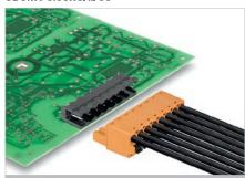
High-temperature-resistant, 90°-angled male header, optimised for SMT processing. The male headers can be manually coded or ordered as pre-coded headers.
