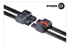
Male plug in 180° outlet direction with PUSH IN spring connection for TNC(S) networks. Also perfect for finger-safe solutions involving inverse voltages. Meets the requirements of UL1059 for 600 V Use Group C. The mating profile ensures touch-safety of > 3 mm in accordance with IEC 61800-5-1.
