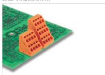
The high-performance device interface with a high connection density. Multi-level PCB terminal with tension clamp spring connection in 5.08 mm pitch for wire cross-sections up to  $2.5\ \text{mm}^2$ .
