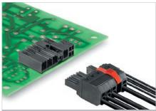
Hybrid male header with 90° outlet direction with power and signal contacts. Fulfils the enhanced requirements for 3 mm of finger safety on 400 V TNC(S) systems in accordance with IEC 61800-5-1 and allows UL approval for 600 V in accordance with UL61800-5-1/ UL840. The self-locking middle flange reduces the space requirements by one pitch width in comparison with conventional solutions.
