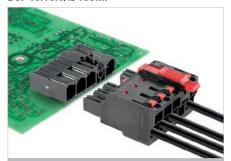
PUSH IN female plug in 180° outlet direction for IT networks. Fulfils the requirements of UL1059 for 600  $\rm V$ Use Group C with leading PE contact when used with SU 10.16IT male header. Fulfils the expanded requirements for 5.5 mm of touch protection (400 V relative to earth), according to IEC 61800-5-1.
