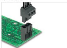
Male header with 180° outlet direction for 400 V TNC(S) systems. Enables UL approval for 600 V in accordance with UL61800-5-1 / UL840. The pin arrangement ensures more than 3 mm of touch-safety in acc. with IEC 61800-5-1.
