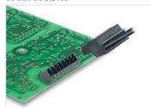
Male header with 135° plugging angle (135° angle between the plugging direction and the solder pin). This corresponds to a 45° angle between the wire orientation and the circuit board.
