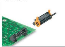
High-temperature-resistant, 135° angled, male header for all common soldering methods in 3.5 mm pitch. 3.2 mm solder pin suitable for reflow and wave soldering. The pin headers provide space for labelling and can be coded.
